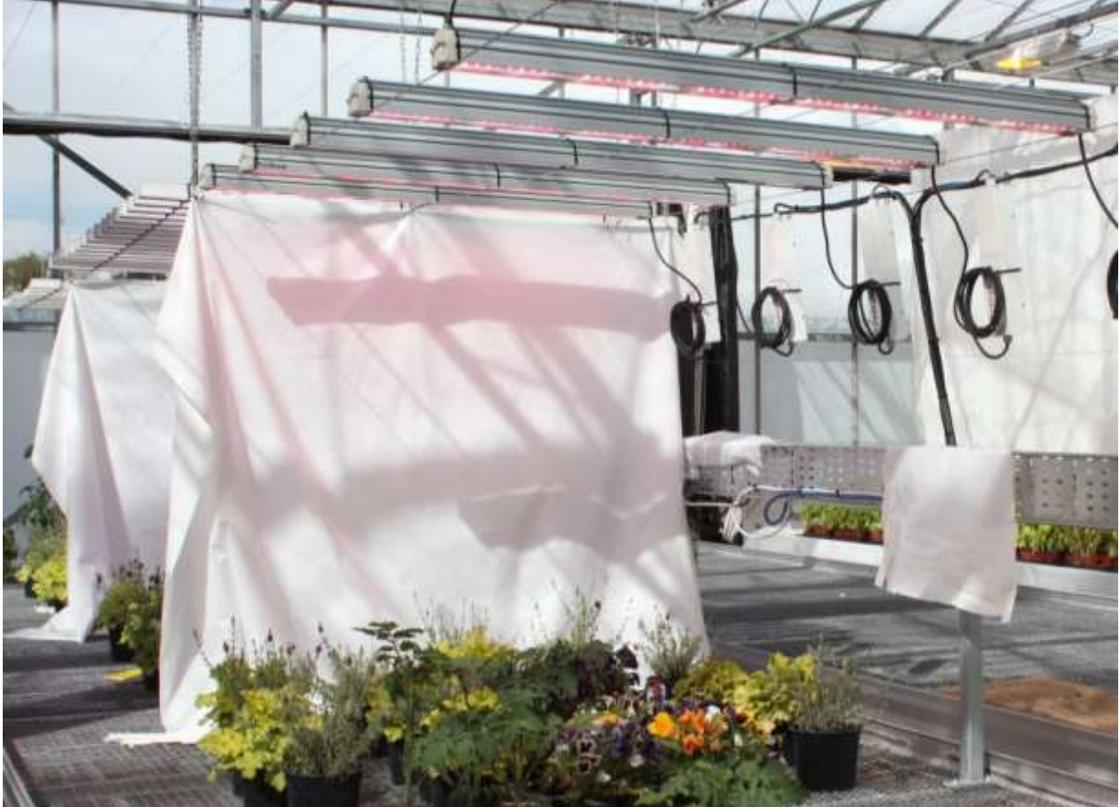
Figure 4.1. Picture of the glasshouse trials with screens in place between the supplemental light treatments.
